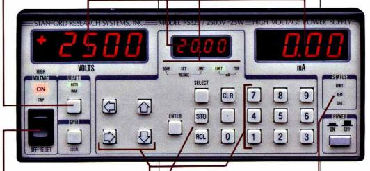
Front panel safety switch enables/ disables the high voltage output and locks out GPIB control.
