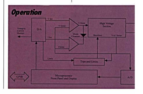
all PS300 Series operation modes remotely. All parameters can be set and read via the interface and Service Requests can be generated in response to overload or trip conditions. A rear panel switch allows the output voltage to be programmed by an analog input voltage and overrides both front panel and IEEE-488 programming.
